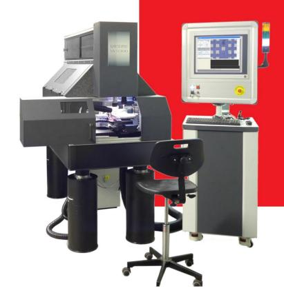
WS-300 is a custom design for an unusual application where exceedingly large depth of focus (up to 3,5mm) was required for processing on steeply curved surfaces. The system combines 1J excimer laser to low Numerical Aperture illumination/homogenisation/imaging optics with a 5m long folded beam path on 2 levels. The WS-300 is vibration isolated and can accommodate various options on stage travel, additional rotational axes etc. Driven by Optec ProcessPower.<sup>TM</sup>
