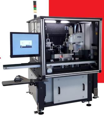
The dual beamwirestripper is a custom design for a precise wirestripping application. 2 optical heads are used at the same time to strip both sides of micro-wires from 30µm to 250µm diameter. The system combines a big excimer laser to a homogenizer and a motorized rectangular aperture mask for stripping size flexibility. Automatic loading/unloading of the part is provided. The machine is fully automated and driven by our ProcessPower<sup>TM</sup> software.
